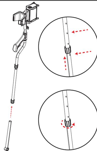
Insert the extension shaft into the upper shaft holding the metal pin pressed and adjust the height by clicking the pin into one of the holes. Then, secure it by tightening the twist lock again.
