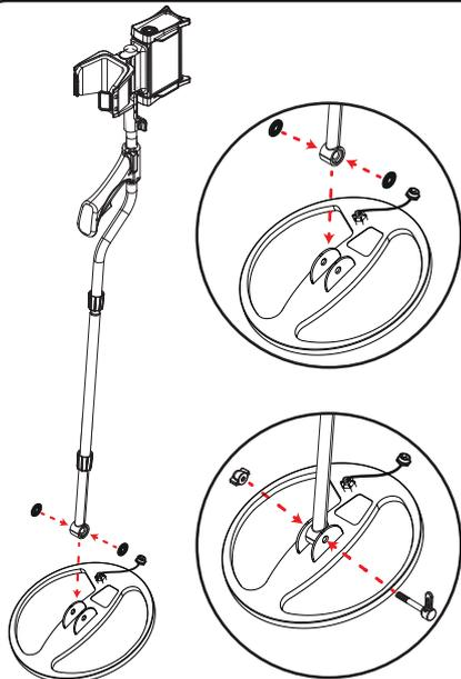
Place the washers into the openings on both sides at the end of the extension shaft. After placing the shaft on the coil as shown in the picture, insert the fastening screw through the hole and tighten it using the wingnut.
