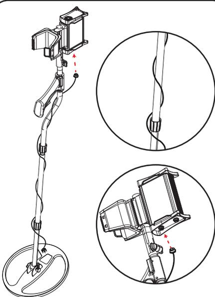
Wrap the coil cable around the shaft all the way up as shown in the picture and after inserting it in the coil input socket underneath the system box, secure it by twisting the connector. Pay attention to not wrap the cable too tight during this step.
