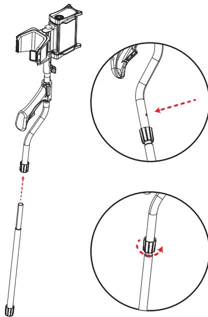
Again by holding the metal pin pressed, insert the upper shaft into the S-rod and click the pin into its hole. Then, secure it by tightening the twist lock.
