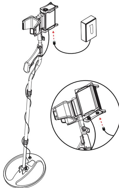
Plug the battery cable into the battery input socket underneath the system box and tighten securely.
