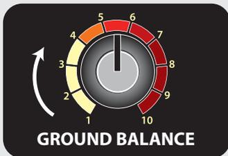
Especially in mineralized ground target signal is negatively affected by the "noise" caused by ground mineralization. This situation may prevent the detector from getting a clean signal from the target necessary for metal detection and accurate discrimination. Ground balancing is a process through which the metal detector is able to cancel out the negative effects caused by ground mineralization.
