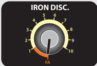
This setting is designed for tough ground conditions and experienced users. For normal ground conditions or if you do not want to bother with this setting it is recommended that you keep it at the factory setting (FS).
